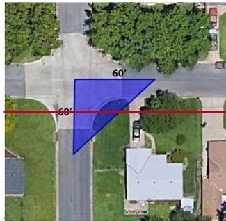
Approach sight triangle. Means a *sight triangle* used for intersection with no control requiring adequate distance for an approaching *motor vehicle* to identify any conflicts in or approaching the intersection before entering.
